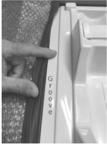
Take the door off and let it warm up to room temperature (72 degrees). Cut the old gasket off the door with a utility knife. This will expose a groove molded into the sides of the door and this is where you will adhere the new gasket. This area should be clean, dry, and free from dust.
